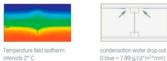
Fig. 11. Thermal insulation of panels with metal-timber beams
